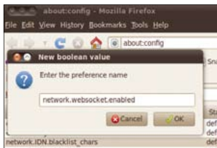
Figure 7: A new Firefox entry in about:config activates the WebSocket API.
